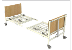
8.2.3 Bring assembled bed halves together
